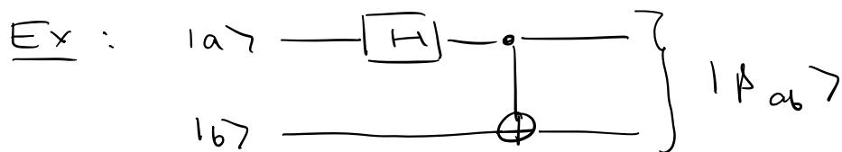
$$\begin{aligned} |\Psi_{ab}\rangle &= \text{CNOT } H \otimes \mathbb{I} \quad |a\rangle \otimes |b\rangle \\ &= \text{CNOT} \quad \frac{|0\rangle + (-i)^a |1\rangle}{\sqrt{2}} \otimes |b\rangle \end{aligned}$$
