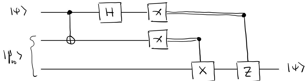
$$\text{det} \quad |\psi\rangle = \alpha|0\rangle + \beta|1\rangle, \quad |\alpha|^2 + |\beta|^2 = 1.$$
